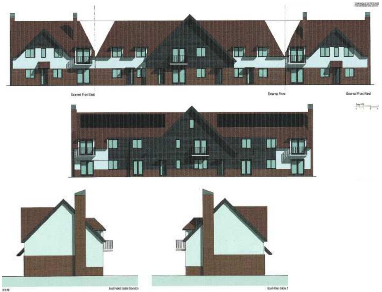
Site D – Apartment building elevations
